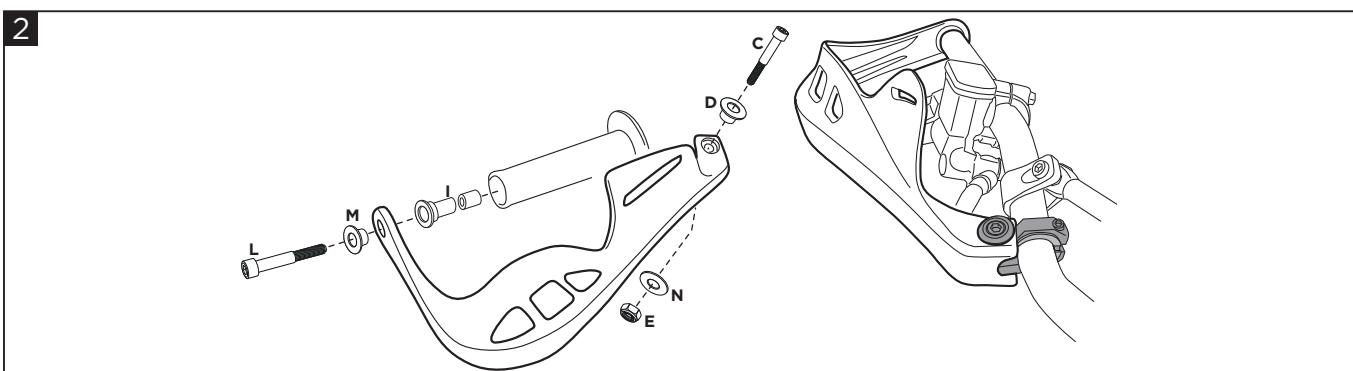
Attach the handguard to the bracelet (A) using the screw (C), the bushing (D), the washer (N) and the nut (E). Attach the handguard to the handlebar using the screw (L), the bushing (M) and the spacer (I).
