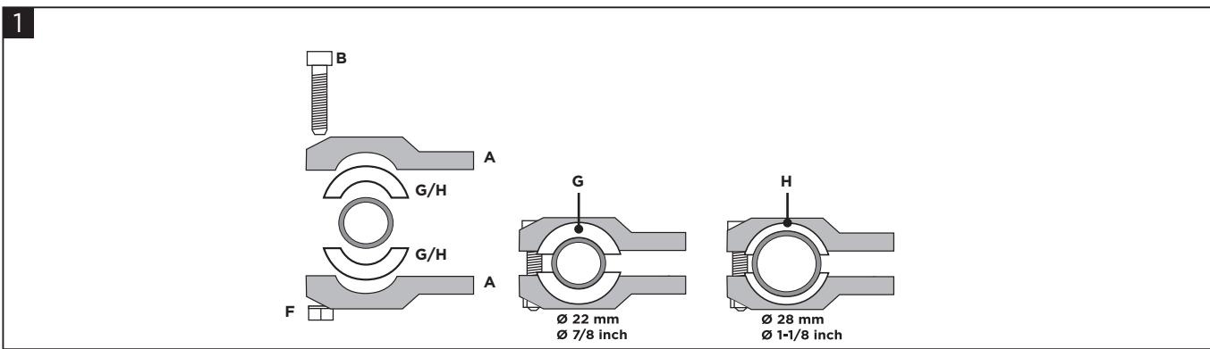
Mount the bracelet (A) on the handlebar using the screw (B) and the nut (F).
